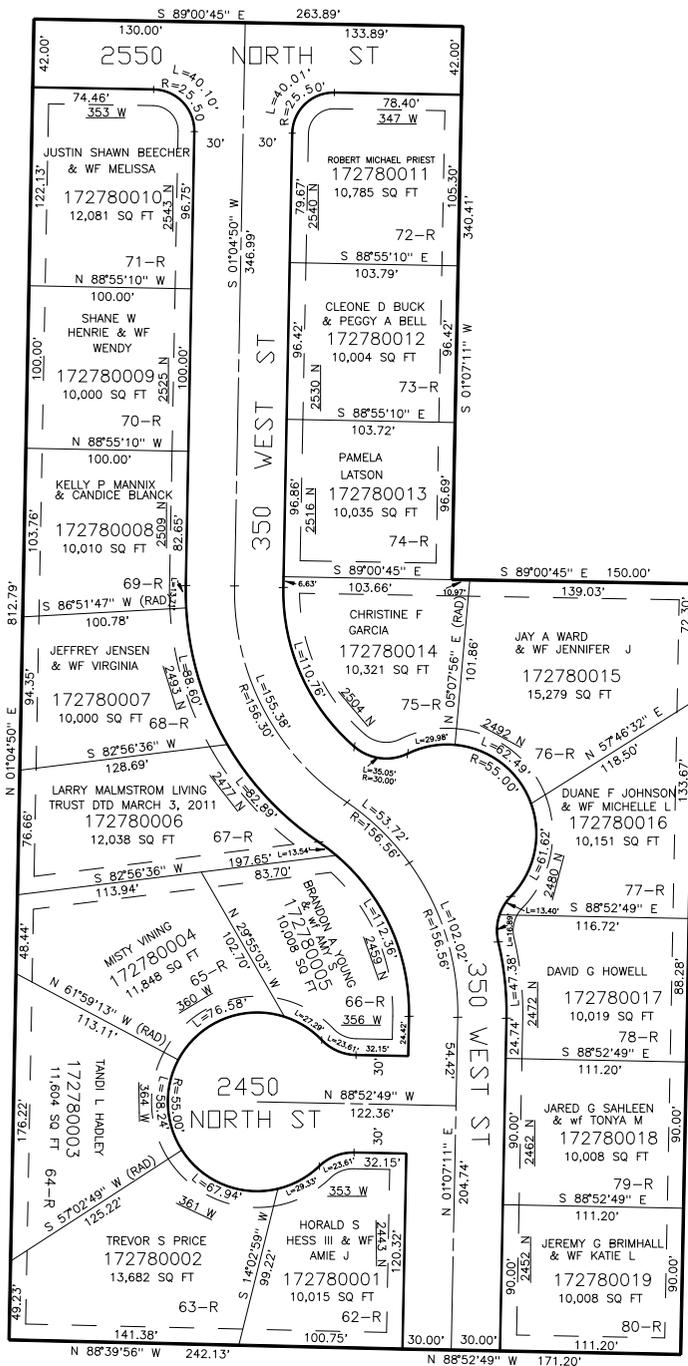
10' UTILITY & DRAINAGE EASEMENTS EACH SIDE OF PROPERTY LINES AS INDICATED BY DASHED LINES EXCEPT AS OTHERWISE SHOWN.
